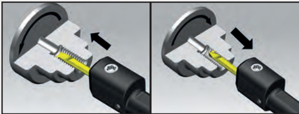
Insert: Right-hand design Direction of rotation: Clockwise M3 turning from outside in Insert: Left-hand design Direction of rotation: Anticlockwise M4 turning from inside out
